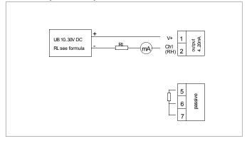
DIC humidity: 0...1 V DC or 0...10 V DC temperature: passive
