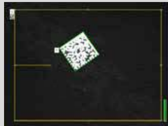
Code reading on solar cells Even extremely small codes (e.g. on silicon solar cells) or highly reflective codes (e.g. on thin-layer solar cells) can be read.
